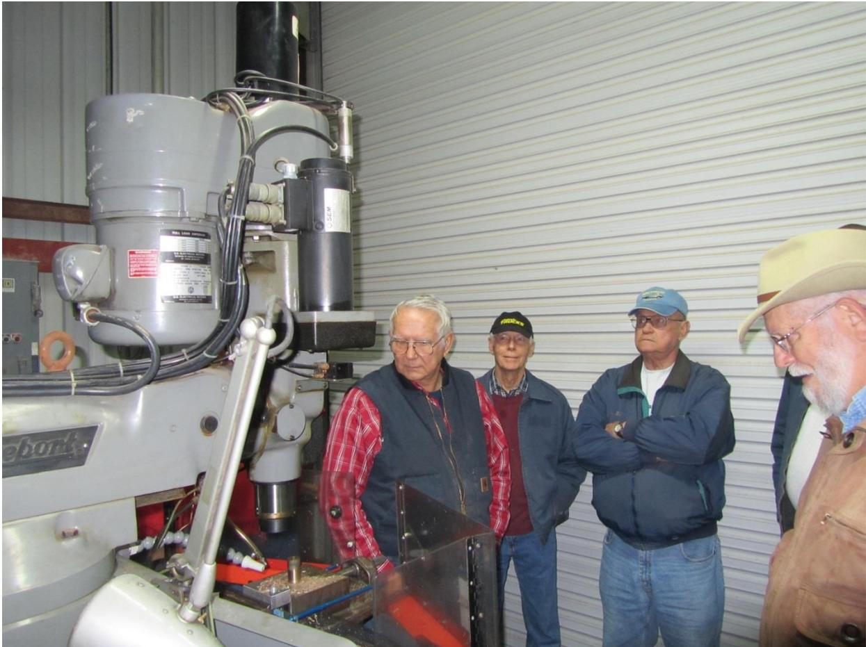
The milling machine was powered up and its features were discussed and demonstrated. Even the software used to control the intricate movements of the cutting tools was revealed. The mood of the group immediately improved. Neil described the machine setup and steps used to complete a project. Recently completed oil pump gears cut from brass round stock were shown.
