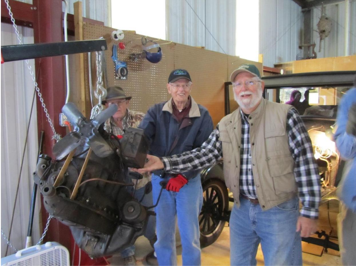
It actually took longer to round up the proper combination of pallets and blocks to position the assembly for separation of the transmission and oil pan. Since we didn't have an engine stand designed to handle the Model T engine, Yankee ingenuity and applied physics were called upon for on-the-spot fabrication.
