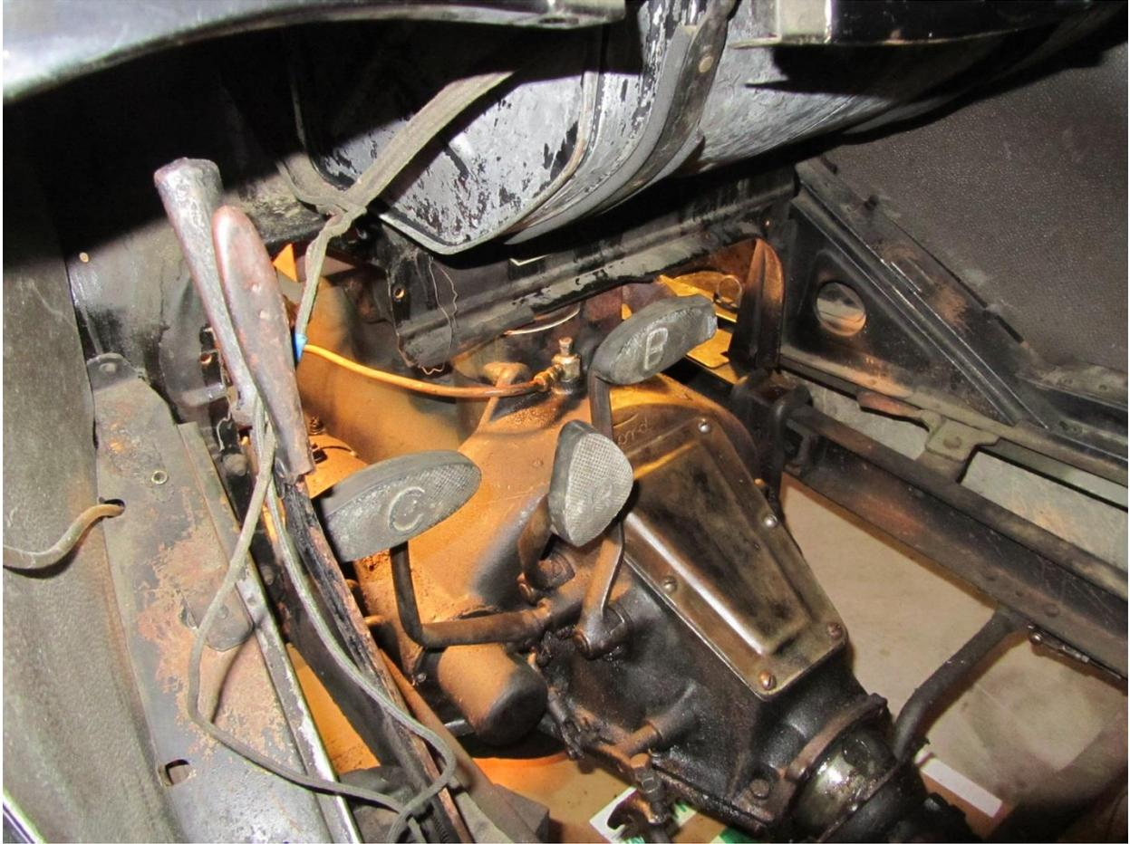
With plenty of willing hands to run the jack and position the engine, the crew pulled the engine forward on the disconnected rear engine mounts. The mounts conveniently slide along the frame rails. Once forward enough, the hoist did the hard work while we steadied and slightly turned the engine with Dan's direction in order for the pedals to clear the firewall.
