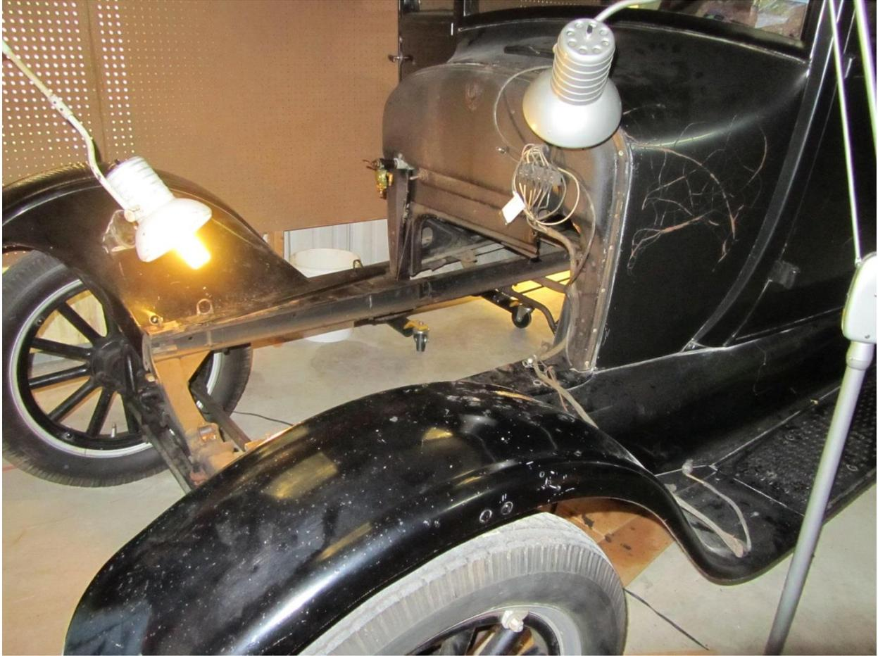
The job has been done correctly when everything that needed to be removed is gone and the remainder is in its place without gouges, bends or dents.
