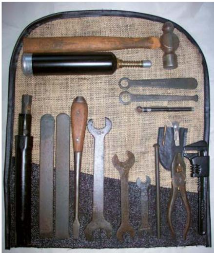
The MG TD tool kit at left is shown with the tools on top of the tool roll which is a reproduction I made. As with the original, it is made of burlap (hessian) that is covered by a black tar like material (I
