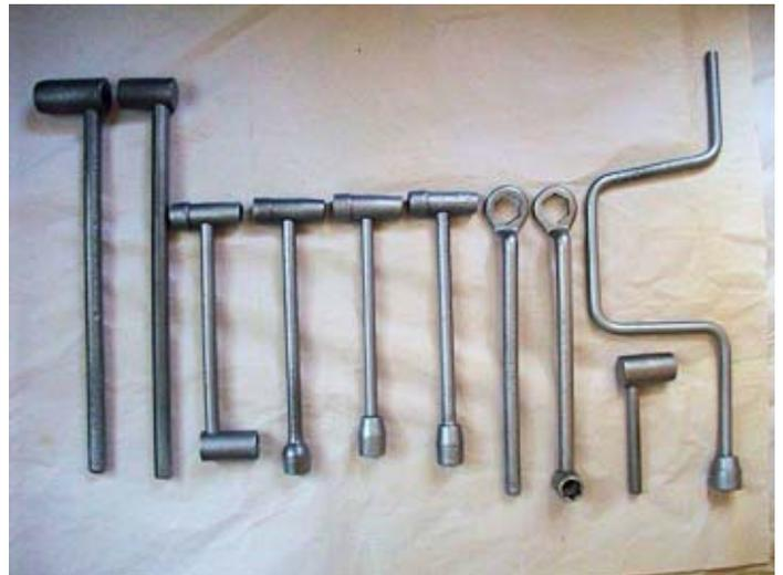
Pictured are some Walden Worcester wrenches I didn't know I had. Eighth wrench from the left is thought to be a headbolt /sparkplug wrench for a Ford model "T". Its marked "3620 Walden Worcester USA Pat Pending 5/8 15/16". While its the correct size, I'm pretty sure there were plenty of Ford script tool kit wrenches to fill the need back in the day.
