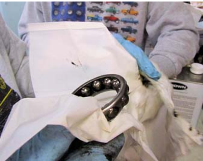
The inner bearing race felt rough to the finger test, but once it was cleaned of grease the reason for the noise was clear. The race had deep galling.
