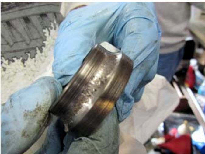
The inner bearing race felt rough to the finger test, but once it was cleaned of grease the reason for the noise was clear. The race had deep galling.
